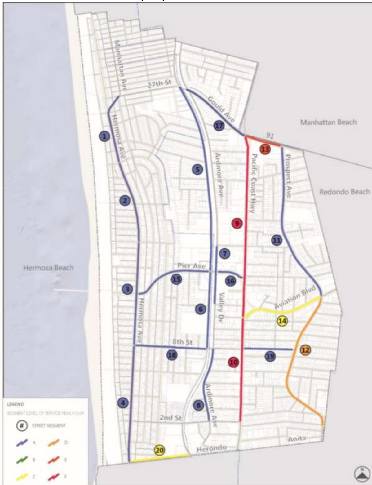
SOURCE: CITY OF HERMOSA BEACH 2015 FIGURE 4.14-9 PLAN HERMOSA (2040) ROADWAY SEGMENT LEVEL OF SERVICE
