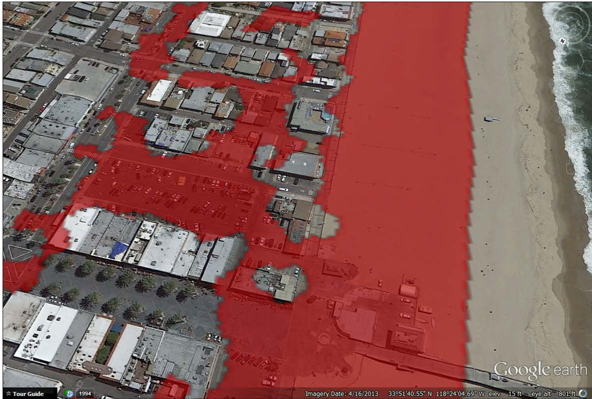
FIGURE 18. OBLIQUE AERIAL VIEW OF AN AREA NEAR THE HERMOSA PIER EXPOSED TO THE 100-YEAR FLOOD WITH 55 INCHES OF SEA-LEVEL RISE. THE AREA IN RED MARKS THE AREA AT RISK OF FLOODING, BASED ON MODELED PROJECTIONS BY THE PACIFIC INSTITUTE (2009).
