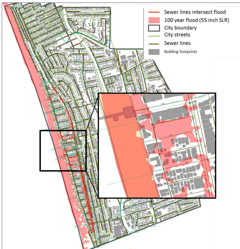
FIGURE 19. SEWER LINES AT RISK OF FLOODING DURING A 100-YEAR FLOOD AFTER 55 INCHES OF SEA-LEVEL RISE (MAIN MAP); AND CLOSE UP OF SEWER LINES IN THE SECTION OF HERMOSA BEACH NEAR THE PIER (INSERT). SEWER LINES WHERE FLOODING IS PROJECTED AFTER 55 INCHES OF SEA-LEVEL RISE ARE HIGHLIGHTED IN BRIGHT RED.
