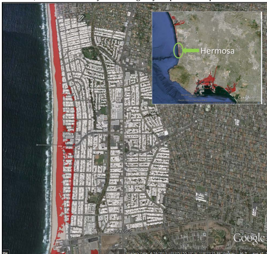
FIGURE 26. EXTENT OF THE 100-YEAR FLOOD WITH 55 INCHES OF SEA-LEVEL RISE (RED) IN HERMOSA BEACH (BUILDING FOOTPRINTS OF CITY IS SHOWN IN WHITE). INSET SHOWS THE EXTENT OF THE SAME FLOOD FOR COASTAL AREAS OF LOS ANGELES COUNTY.
