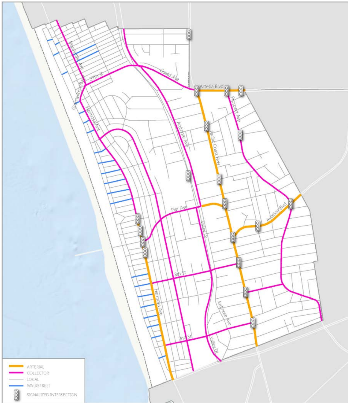
FIGURE 17.1: HERMOSA BEACH STREET CLASSIFICATION AND SIGNALIZED INTERSECTIONS
