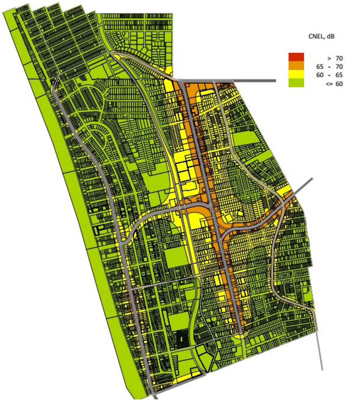
Figure 6.7 Future (2040) Noise Contours in the City of Hermosa Beach with PLAN Hermosa
