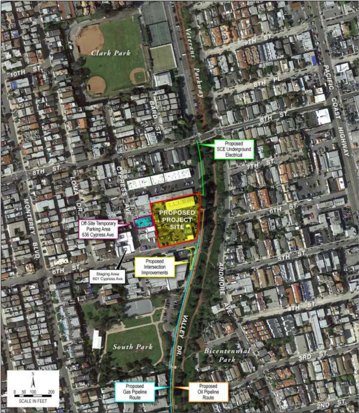
Figure 2.5 Project Site and Pipeline/Electrical Connections
