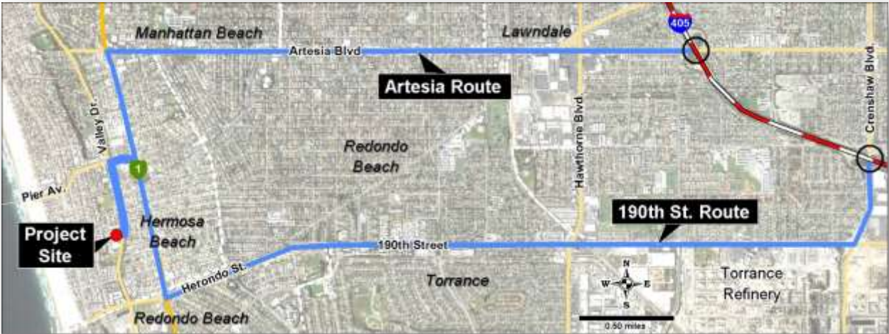
Figure 2.12 Truck Routes from Highway 405 to Project Site
