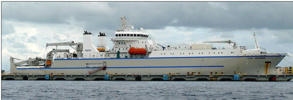
Figure 2-10. Typical Cable-Laying Vessel
