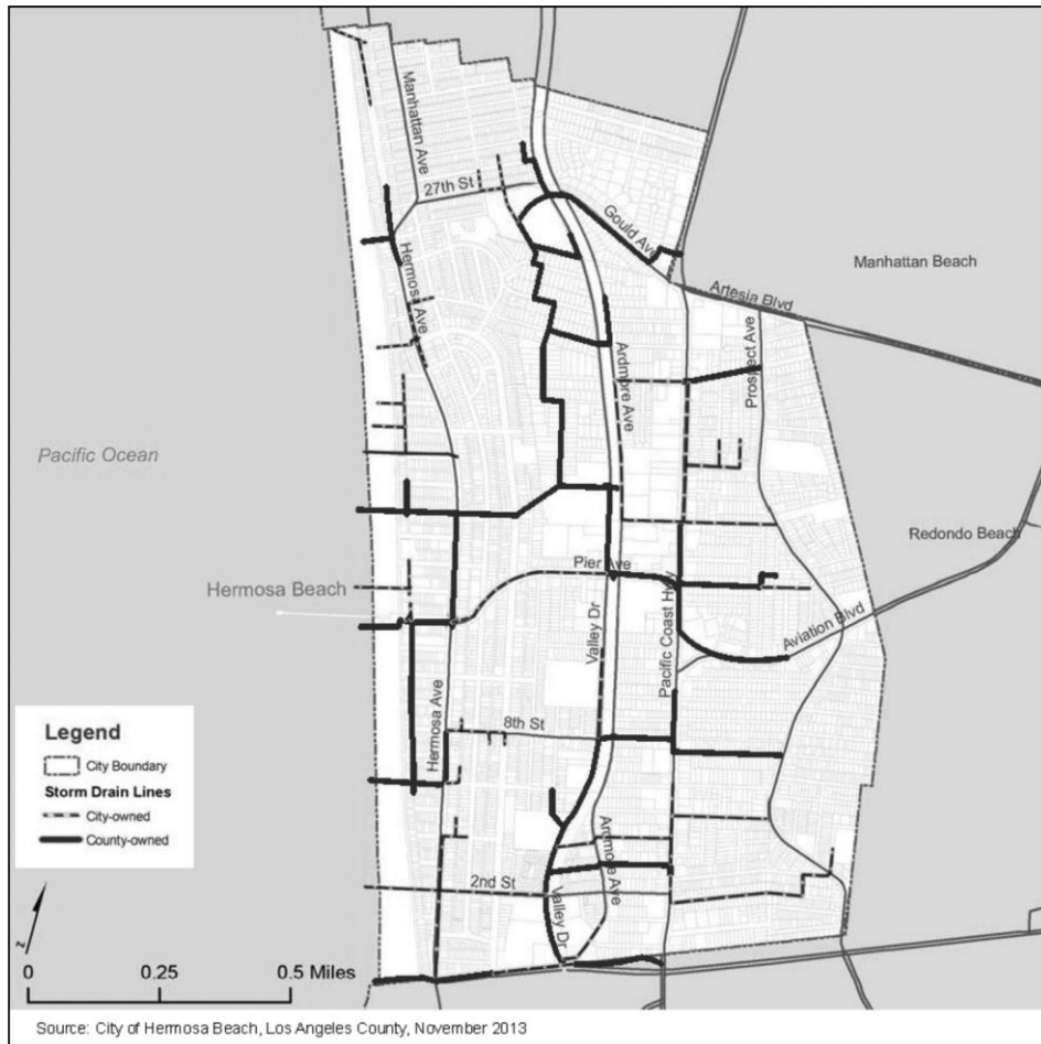
Figure 3.8-1. Stormwater Drainage Map
