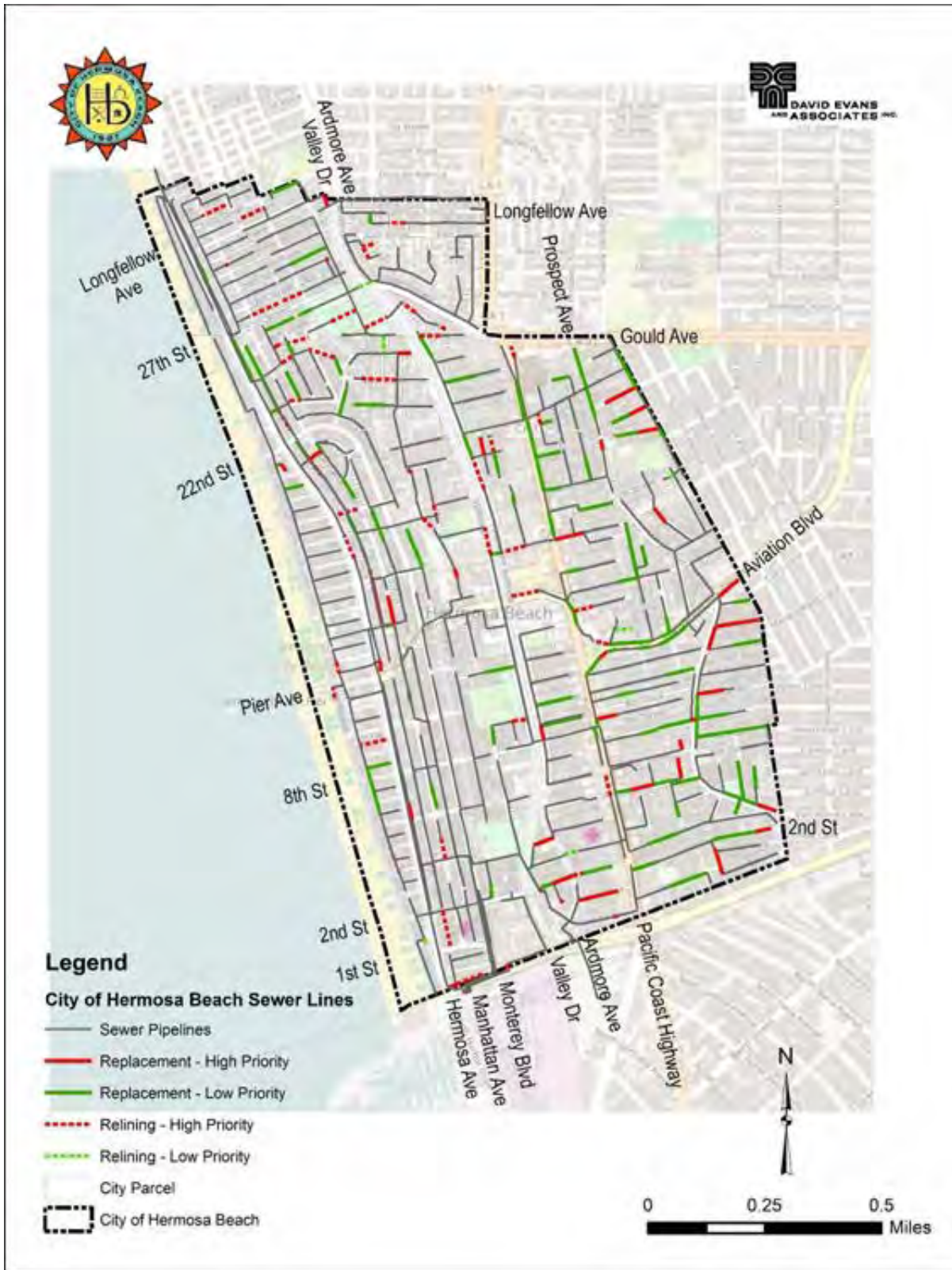
Figure 5-3: Sewer System Defects Recommended for Rehabilitation
