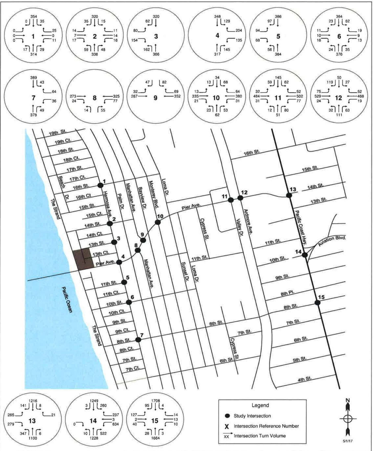
Figure 4.19 Existing With Project Traffic Volumes - Saturday – Midday Peak Hour Pier and Strand Hotel - Traffic Study
