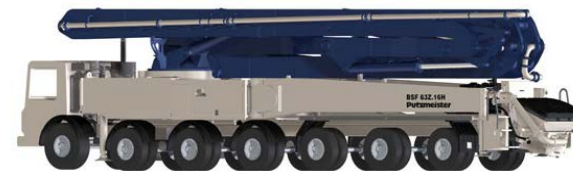
Concrete Pumping Truck 77,000 lbs. loaded - 43' long
