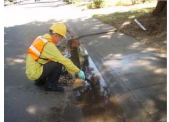
Figure D-3 Measuring pH and turbidity in-stream measurements
